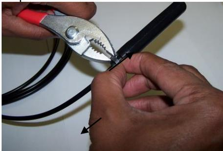
4. Carefully remove the Cover by pulling it away from the Plug. Rock the Cover back and forth to ease removal.
