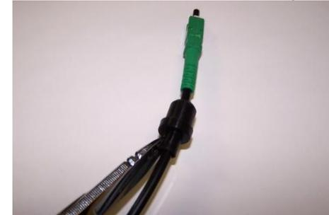
6. Remove the Plug from the cable.
