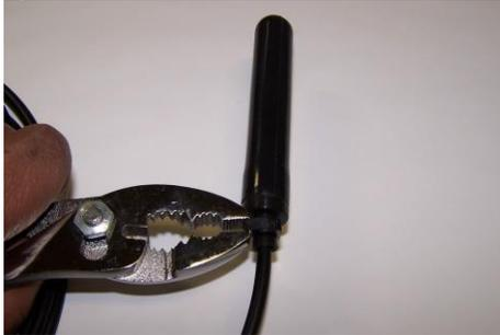
3. Grab the other side of the Hose Clamp latching feature and pull the latches laterally apart, to release the Hose Clamp. Remove the Hose Clamp from the cable.
